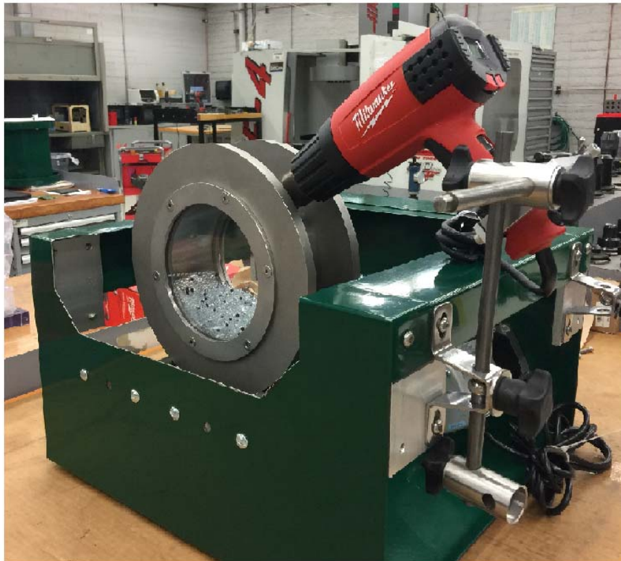
Experimental setup: Rotating stainless steel drum with heat gun to heat the drum walls
